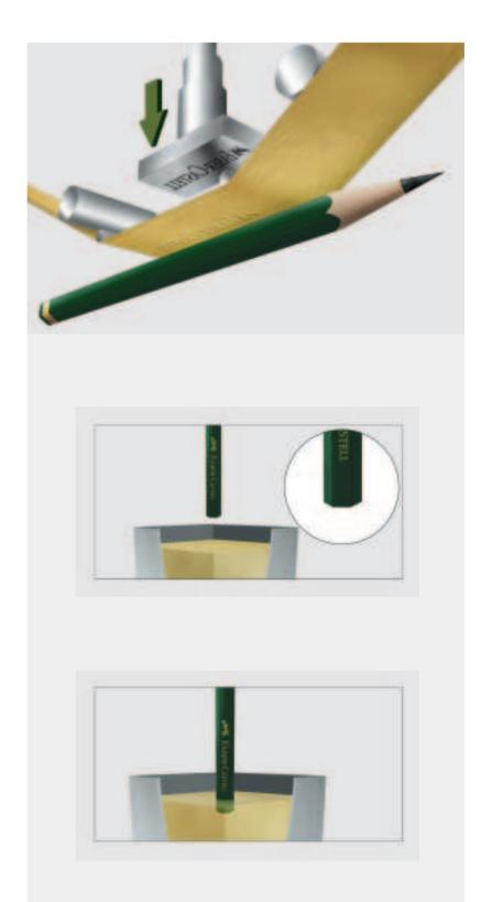
THE PENCIL IS INITIALLY DIPPED INTO A PAINT BASIN TO A SPECIFIED DEPTH.
