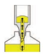
For the refill process, too, the capillary effect is utilised. The ink automatically rises from the ink-pot through the capillaries of the tip into the Textliner and can be used again soon afterwards. Overfilling the Textliner is not possible as it only accepts as much ink as has been depleted from its reservoir.
