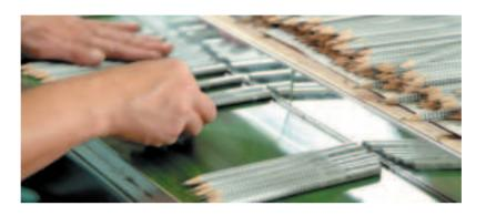
The pencils are checked after each production stage, e.g. for breaking strength, sharpenability and hot-foil stamping. Any pencil failing these controls is rejected.
