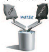
Finely ground graphite and purified clay are mixed in accordance with precisely specified, designated formulas.
