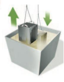
drying process, the raw leads are fired for one hour at 900° C. In the final finishing step the now porous leads are soaked in a grease/wax bath. That is how the leads obtain their specific writing quality.
