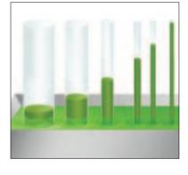
An absorptive reservoir made of synthetic fibres consists of a tube system storing the writing fluid. During the writing process, ink is continuously fed to the paper and since the narrower cavities in the tip cause a
